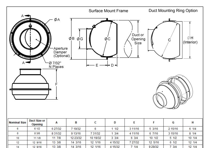
Designed to handle large air capacity requirements and provide concentrated long throws.
